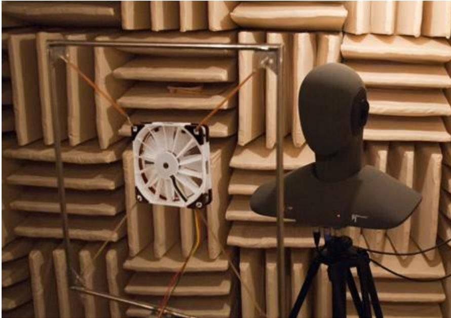
*Prototype of a Noctua NF-F12 fan with integrated RotoSub ANC technology during acoustic tests in an anechoic chamber.*
